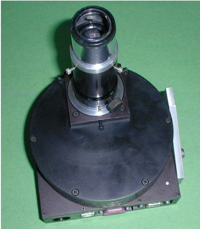
Figure 4: Coronagraph Attached to ST-7 CCD.
